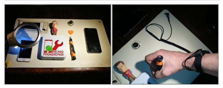
• Using your <u>Anti-static mat</u> and wristband correctly.
