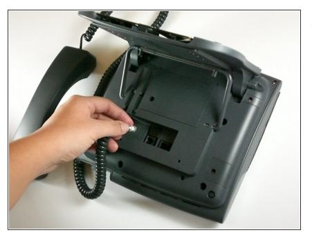
Before disassembling the phone, make sure it is not plugged into power and the handset phone cord is disconnected from the handset jack.
