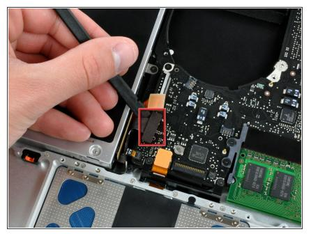
Use the flat end of a spudger to pry the hard drive cable connector straight up off the logic board.
