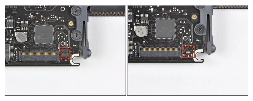
Some 2.0 GHz A1278 MacBook Unibody logic boards do not have the necessary socket installed to accept the keyboard backlight ribbon cable attached to the upper case. The first and second pictures show logic boards with and without the socket installed, respectively. If your logic board does not have the backlight ribbon cable socket installed, the keyboard will work but the keys will not light up.
