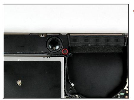
Remove the single Phillips screw securing the subwoofer to the upper case.
