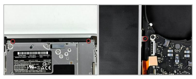
Remove the three 2.5 mm Phillips screws securing the optical drive to the upper case.
