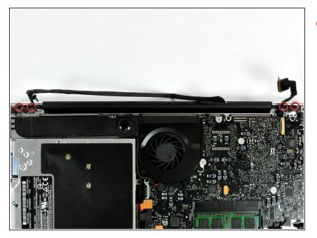
Remove the two outer 6 mm Torx screws securing each side of the display to the upper case (4 screws total).
