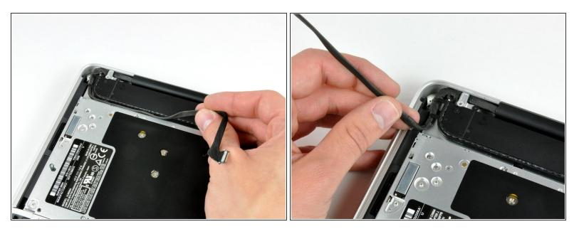
• De-route the camera data cable from the channel in the optical drive.
