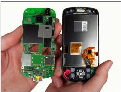
Gently lift the motherboard out of the front enclosure once the screws are removed.
