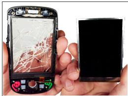
Gently pry out the LCD screen from the left side of the enclosure as illustrated, using an plastic opening tool.
