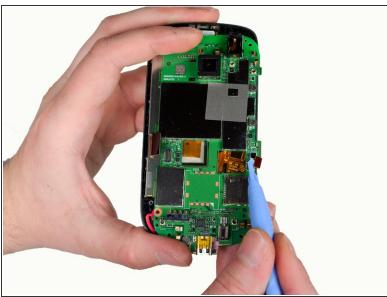
Gently release the two ribbon cables using a plastic opening tool by prying up the pop connectors used to attach the ribbon cables to the motherboard.
