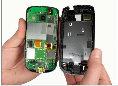
• Carefully separate the front and back enclosures once all of the clips have been disengaged.
