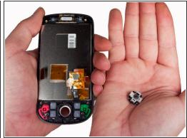
(i) Remove the trackball and its enclosure by turning the phone over into your cupped hand and allowing the trackball and enclosure to fall out.
