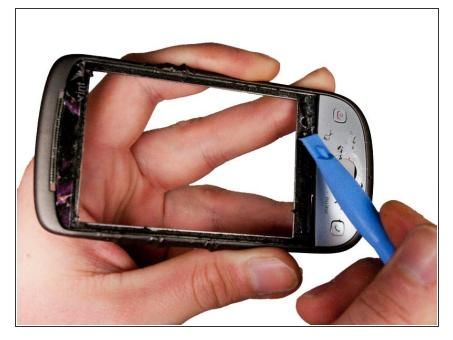
Remove any excess adhesive from the plastic frame.
