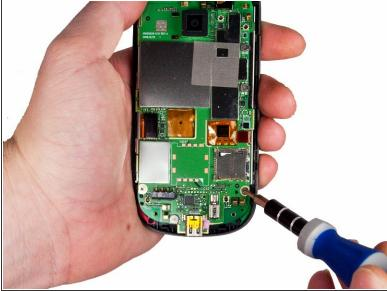
Remove the two screws located at the bottom left and right of the motherboard using a small Phillips screwdriver.
