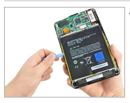
Repeat the process from the previous step to free the left battery cell.
