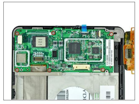
Remove the six 2.6 mm Phillips #00 screws securing the motherboard to the frame.
