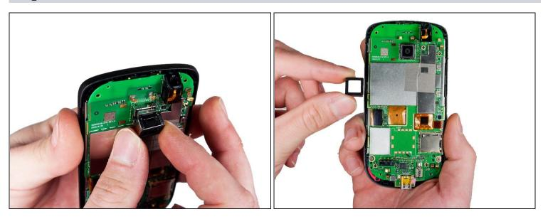
• Pull the released camera enclosure away from the motherboard until it is completely free.
