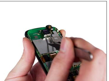
• Using a pair of metal <u>tweezers</u>, simultaneously depress both tabs on one side of the camera enclosure and **gently pull up** until tabs come free. Repeat for the opposite side.
