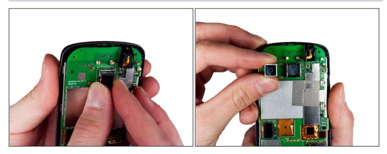
• Now with camera unit exposed, **gently wiggle the camera** as you pull away from the phone to remove it.
