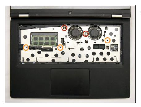
Locate and remove the screws holding the bezel to the laptop body:
