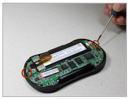
• Unscrew the 2 Philips #00 screws on each end of the motherboard.
