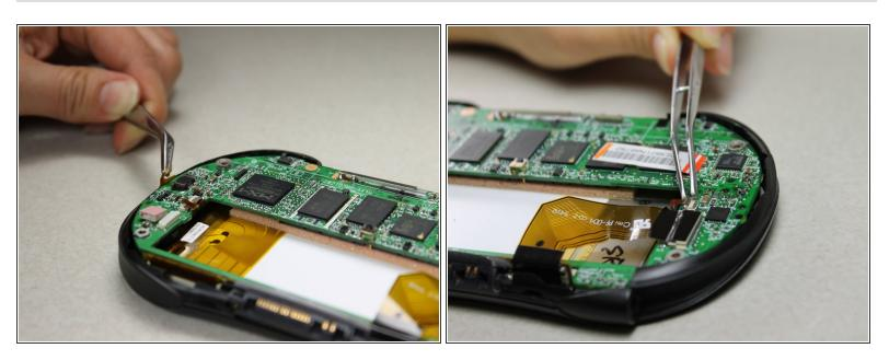
Disconnect 2 brown wire-tape ends from each end of the motherboard. Gently pull straight out with tweezers.
