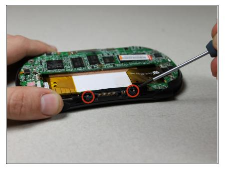
• Unscrew the 2 Philips #00 screws on each side of the charging port.
