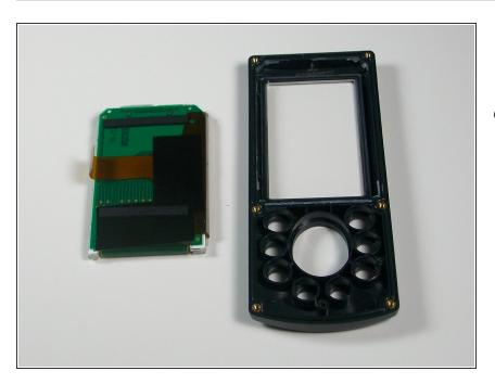
With the display removed, the front case of the Garmin GPS can be replaced.
