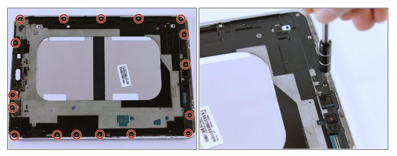
• Remove all seventeen 3 mm screws using a PH000 Phillips screwdriver.
