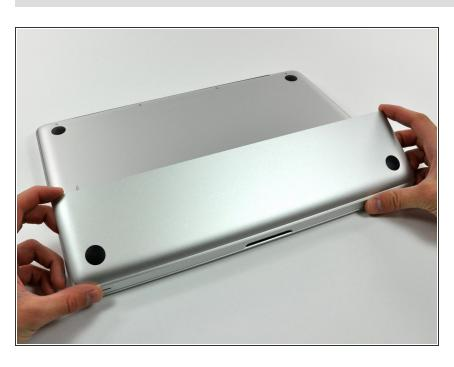
The access door should now be raised enough to lift it up and out of the Unibody.
