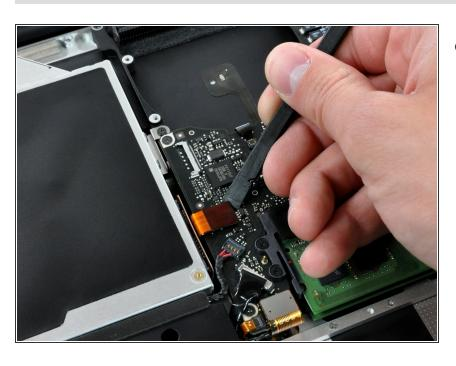
Use a spudger to carefully pry the optical drive connector straight up off its socket on the logic board.
