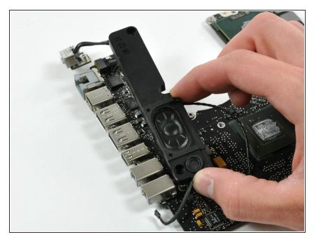
Lift the left speaker assembly out of the logic board.
