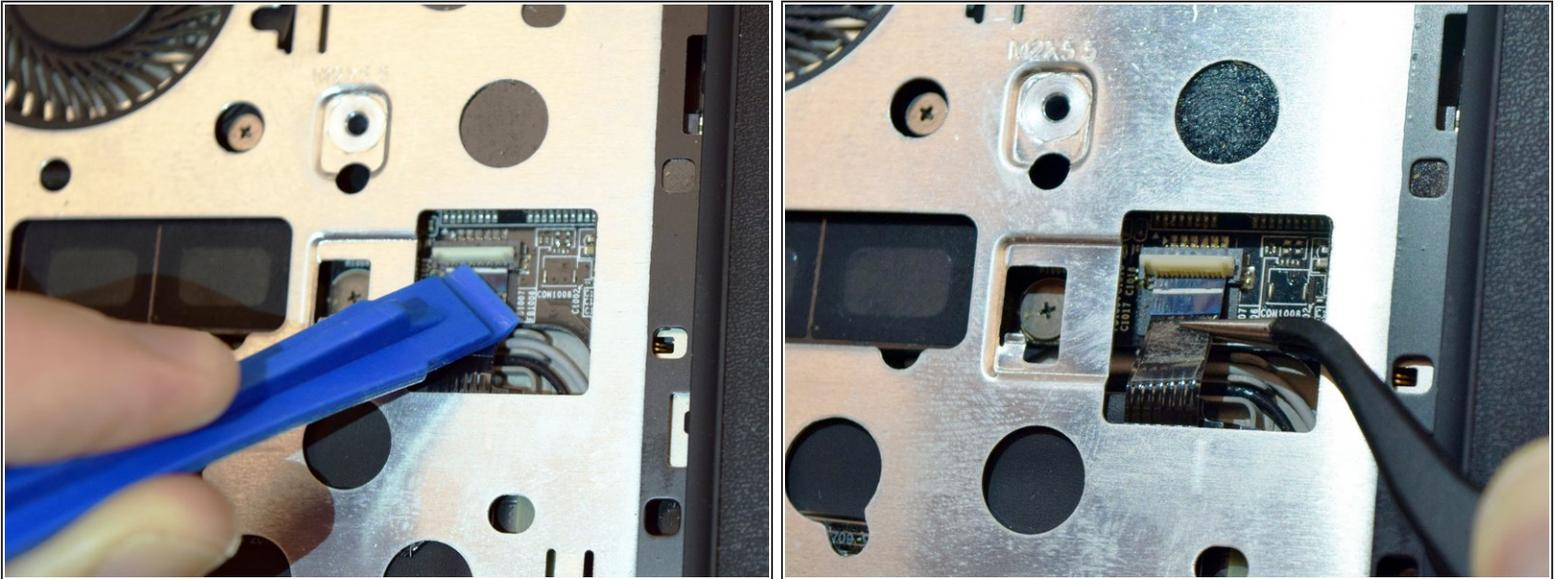
**!** There is now nothing securing the bezel to the laptop body. However, there are still two cables connecting the bezel to the mainboard. Ensure the bezel remains in place until the cables are disconnected.
