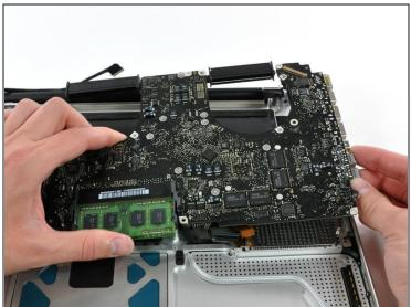
• Carefully lift the logic board assembly from the left side and work it out of the upper case, minding the port side that may get caught during removal.
