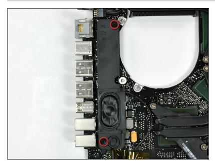
• Remove two 5 mm Phillips screws securing the left speaker to the logic board.
