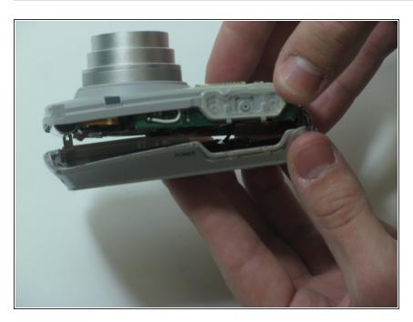
Carefully separate the front and back of the camera
