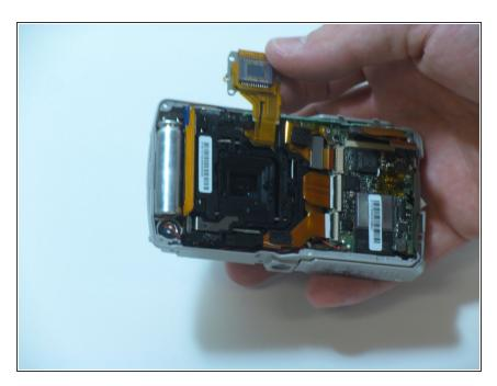
Remove the larger black rubber frame. Clean with condensed air.
