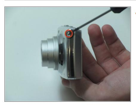
Remove the screw located on the right side of the camera
