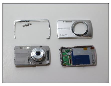
i You should be left with 4 large pieces, the outer case, inner lens piece, outer silver band and back case containing the LCD display.
