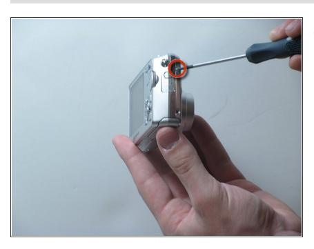
Remove the two screws from the left side of the camera
