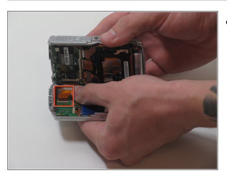
Carefully flip up the clip attaching the ribbon from the rear to the front and pull it out
