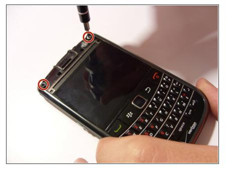
Using a T6 Torx screwdriver, remove the two screws from the top corners of the device.
