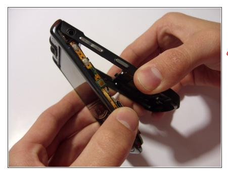
• Remove the back chassis by gently pulling the chassis back and forth.
