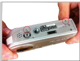
Remove the four screws from the casing.
