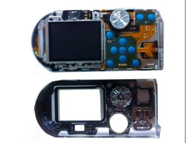
Carefully pull the back casing away from the camera.
