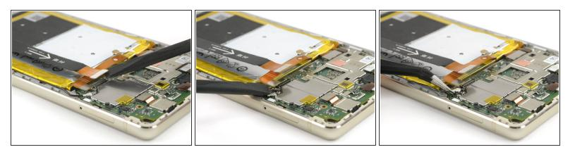
Disconnect the motherboard flex, the battery flex and the antenna cable.
