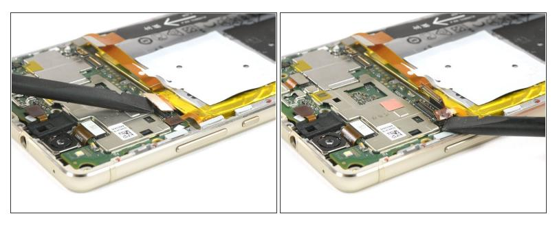
• Disconnect the display flex and the power and volume button cable.
