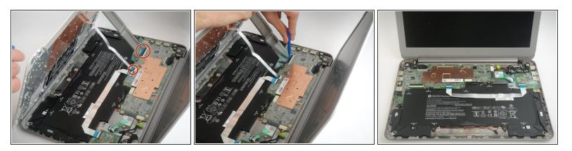
Using a plastic opening tool or your fingers, lift the two black flaps that hold the ribbons connecting the keyboard and touch-pad to fully disconnect the keyboard from the laptop.
