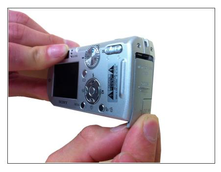
Pull the battery cover in a downward motion, following the arrow on the cover, until it is released.
