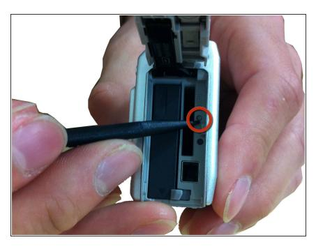
Locate the reset button near the battery compartment and push the button with a pointed object such as a paper clip or pry tool.
