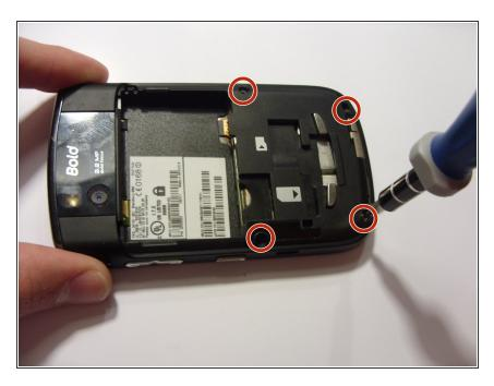
Using a T6 Torx screwdriver, remove the four screws from the bottom half of the device.
