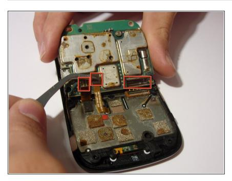
Using a pair of tweezers, remove the three ribbon connectors.
