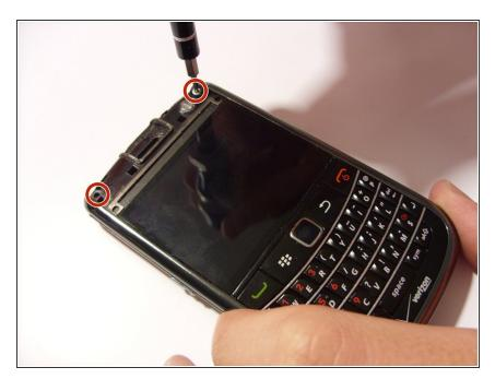
Using a T6 Torx screwdriver, remove the two screws from the top corners of the device.
