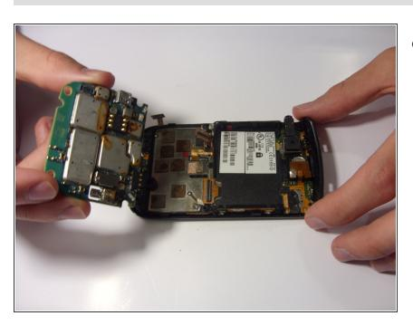
Remove the mother board by lifting the board upward.
