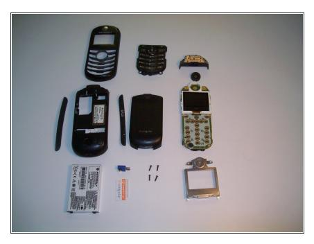
List of Parts: Battery, SIM Card, Vibration mechanism, back cover, Front Case, Back Case, 2x rubber sides, 4x Screws, Antenna, Speaker, Keypad, Metal screen cover.
