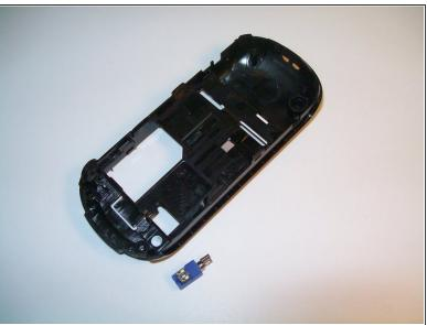
Using your hands or the pry tool, gently lift the vibration mechanism out of the rear casing.
