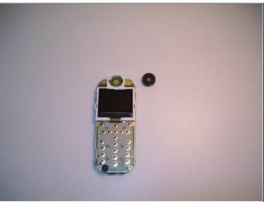
Lift to remove the speaker from its contact point on the logic board.
