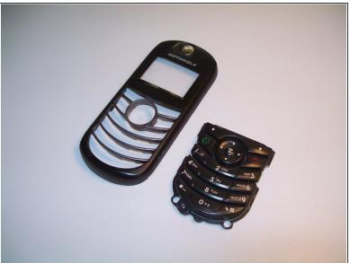
On the top half of the phone push downwards on the number keys to free the keypad from the top of the phone.
