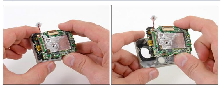
• Gently grab the edges of the motherboard assembly and lift it out of the front case.
