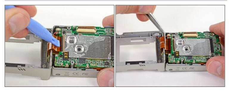
• Using a plastic opening tool or your fingernail, flip up the locking tab on the SD board ribbon cable ZIF connector on the motherboard assembly.
