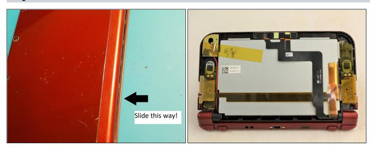
• From the hinge, slide the outer portion of the top shell so that it separates from the inner portion.
