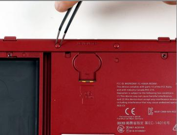
Using <u>tweezers</u>, carefully pop out the rubber bumpers located at the top side of the 3DS.
