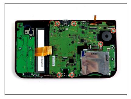
Using a JIS #000 screwdriver, remove six 4mm screws along the edges of the motherboard.
