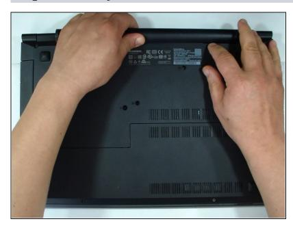
Switch off the laptop, disconnect the AC adapter, and remove the battery.
