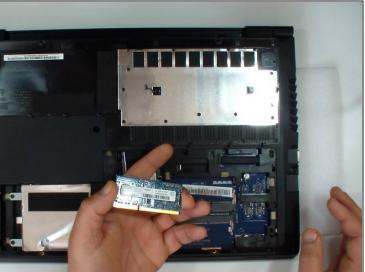
• To pop up the memory module you'll have to spread latches on both sides of the slot.
