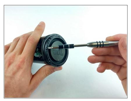
Go around the outer edge of the side passive driver with a screwdriver to remove the seven 8.9mm Phillips #00 screws from both sides of the device. Make sure to set the screws aside somewhere they won't get lost.
