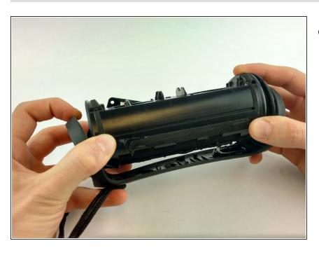
Use your hands to carefully remove the outer frame to expose the inner components of the speaker.
