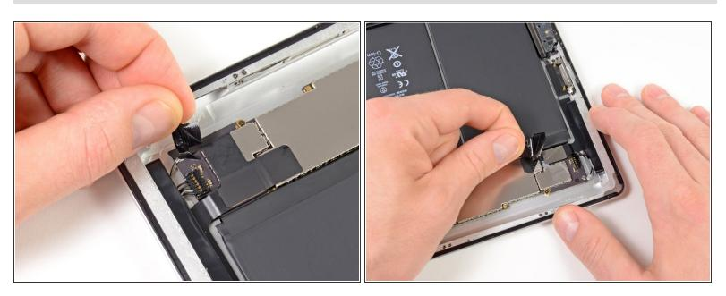
if present, remove the pieces of electrical tape covering the Wi-Fi antenna, speaker cable, and dock connector cable.
