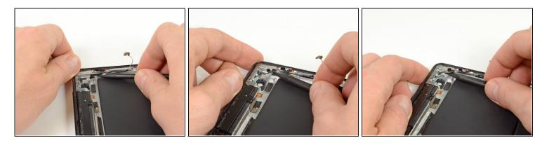
• Continue sliding the tip of the spudger toward the top of the iPad, releasing the adhesive.
