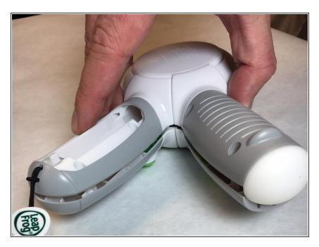
Separate the top and bottom parts of the controller slightly.
