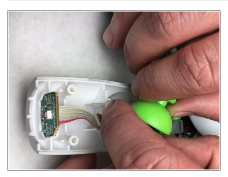
Hold the circuit board and button and pull the button off.
