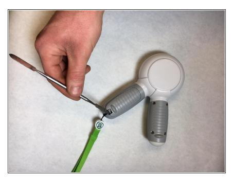
Use the Metal Spudger to push the release clip on the battery cover.
