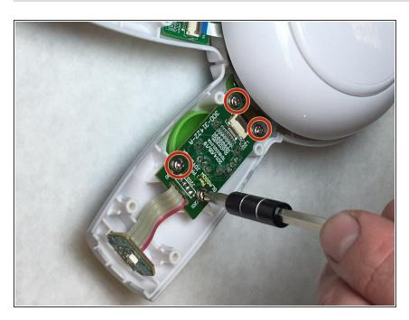
Use the screwdriver to remove the four 8.7 mm PH1 Phillips head screws.
