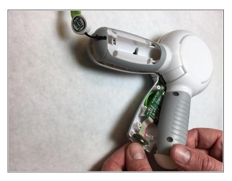
Slide the cover on the back side of the controller covering the joy stick out of the way.
