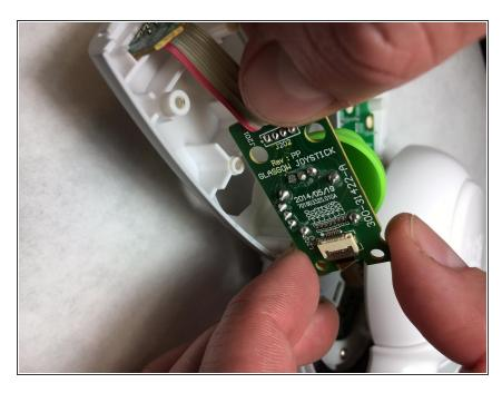
Turn and lift the circuit board with button attacked out of the hole. Do not detach the circuit.
