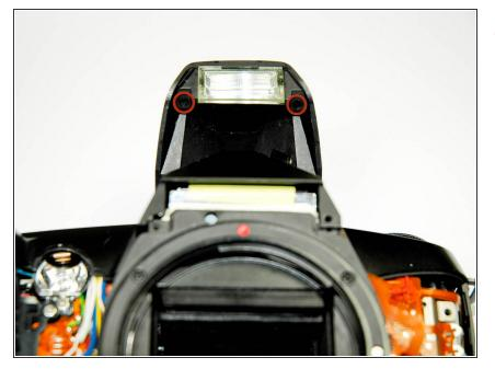
• Unscrew the two screws on the front of the flash near the bulb cover.
