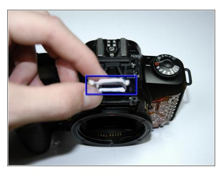
Remove white cocking with a razor blade, and then unsolder connection.
