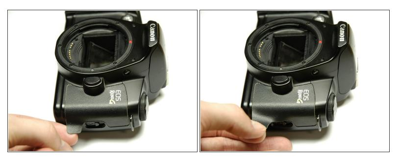
• Using your finger, peel back the textured grip so the components are separated.
