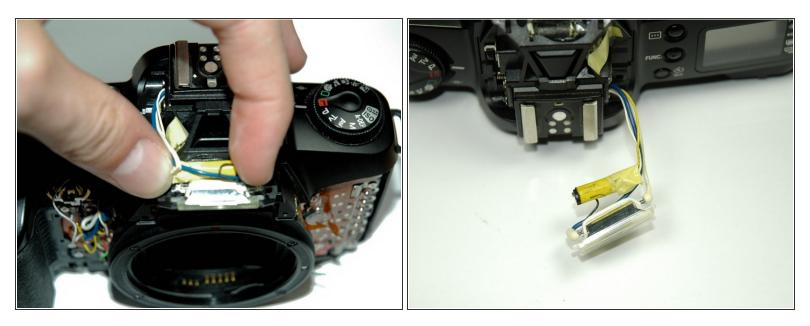
• Pull off yellow capacitor from flash wiring.
