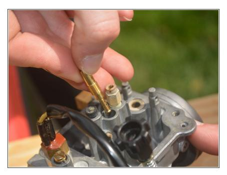
Use a flat blade screwdriver to unscrew and replace the carburetor jet provided in the carburetor kit.
