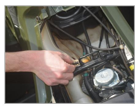
Remove the plastic rivet that connects the air-intake tube to the metal frame of the four wheeler.
