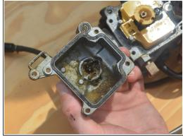
Use a Phillips screwdriver to remove the four screws that secure the float-bowl assembly.
