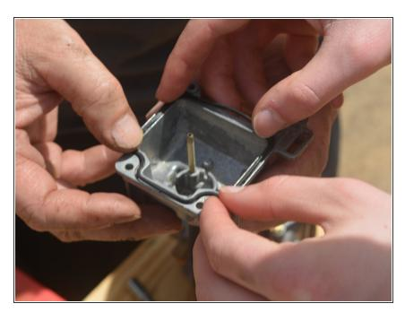
Remove the old gasket from the float bowl assembly and replace it with the new gasket provided in the kit.
