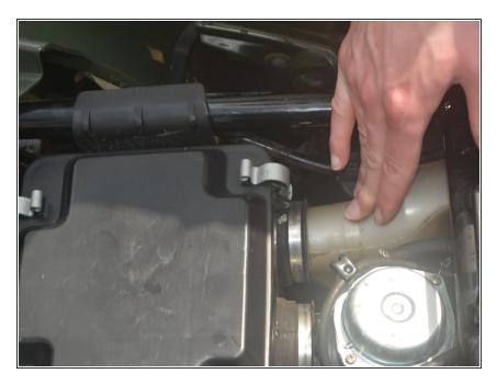
Pull the air-intake tube backwards away from the air filter box.
