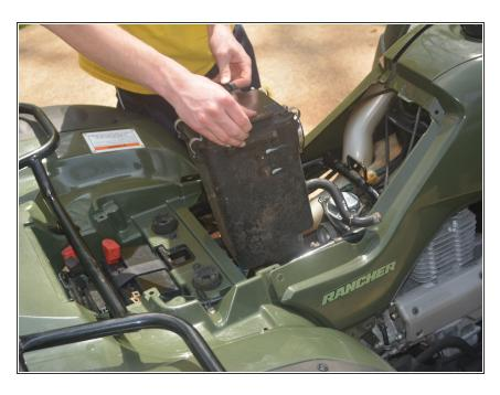
At this point, the black air filter box should be loose. Lift the air filter box vertically out of the four wheeler.
