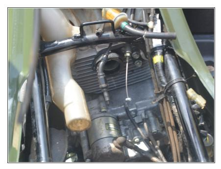
At this point, the carburetor should be fully disconnected. Lift the carburetor up out of the four wheeler and gently place it on a table where it can be further disassembled.
