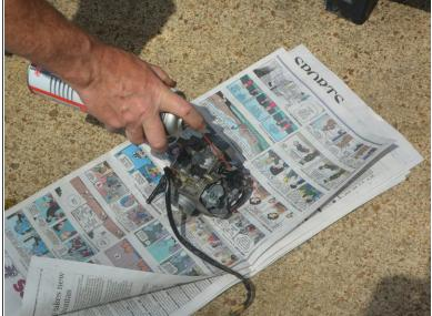
• Thoroughly spray carburetor cleaner all over the outside, inside, and openings of the carburetor.
