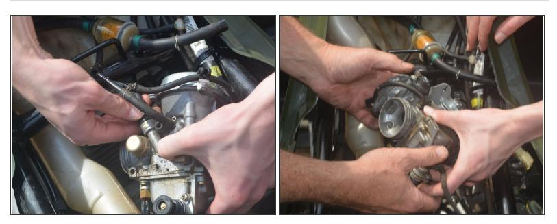
Remove the choke cable attached to the carburetor by twisting the carburetor around to unscrew it.
