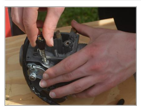
Unscrew and replace the idle speed adjustment screw and spring provided in the carburetor kit.
