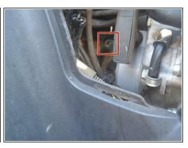
Use a 10 mm socket wrench to remove the screw on the right hand side of the bottom of the black air filter box.
