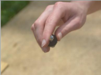
• Use a T30 Torx screwdriver to remove the screw securing the black plastic panel on the left side of the four wheeler.
