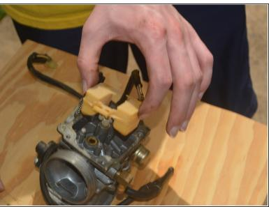
Use a punch or small flat blade screwdriver to drive out the pin holding the float and lift the float out.
