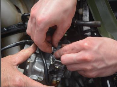
Twist the spring-loaded mechanism located underneath the black cover that was just removed in the previous step in order to loosen and slip the throttle cable out of the inside of the carburetor.
