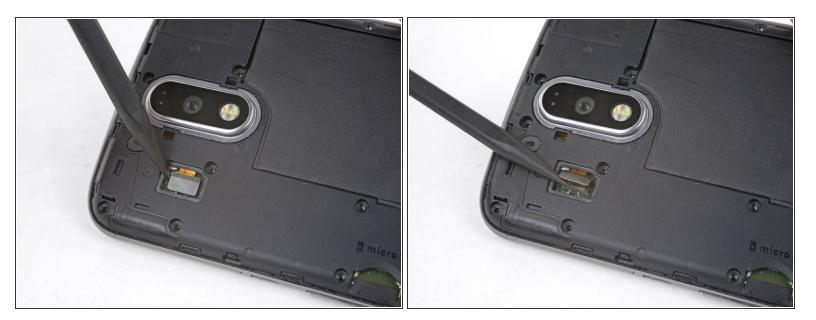
• Use the point of a spudger to pry up and disconnect the camera flash connector.
