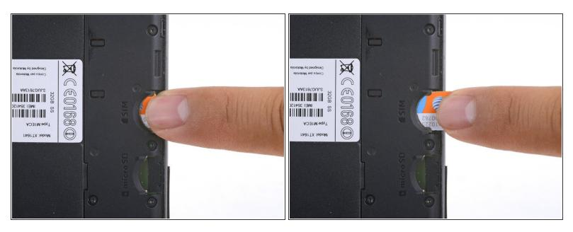
• Slide out and remove the SIM card.
