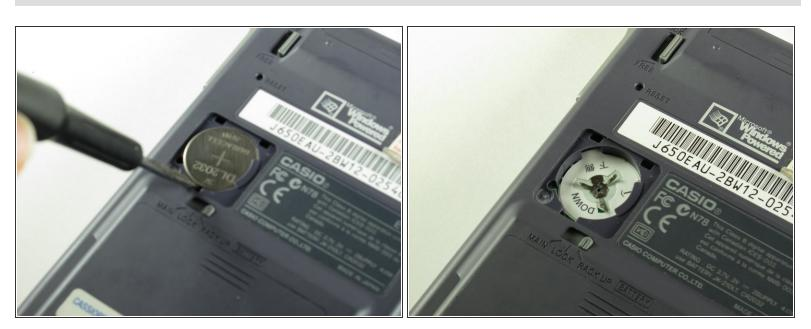
• Insert a Spudger underneath the battery and pry upward to remove it.
