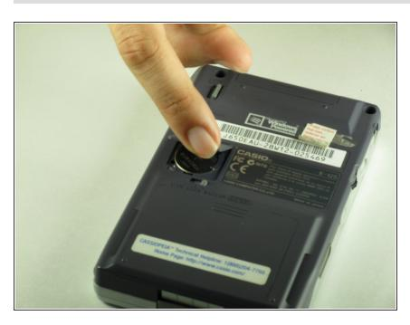
Remove the battery cover by pulling bottom section upwards as shown.
