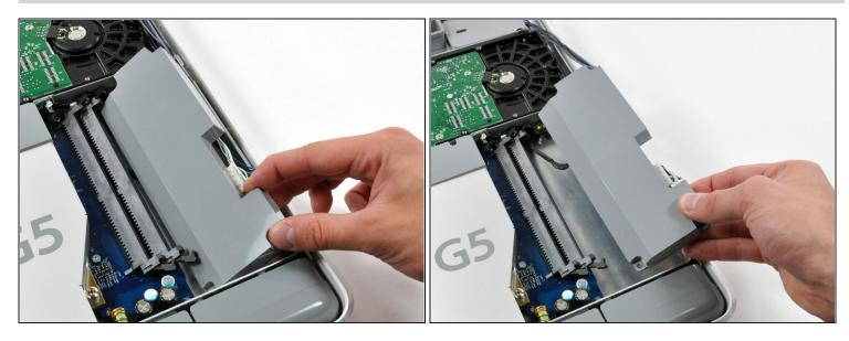
• Slide the inverter toward the edge of the mid-plane, then lift it out of the iMac.
