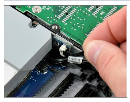
• Disconnect the hard drive thermal sensor cable from the thermal sensor board on the hard drive bracket by pulling the cable away from the heat sink.
