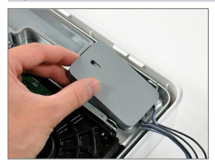
• Flip up the inverter cable cover from its left edge and lift it out of the chassis.
