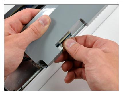
• Disconnect the small inverter cable connector by pulling it straight away from its socket.
