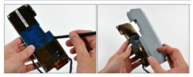
If you wish to replace just the inverter board, use a spudger to pry off its plastic cover.
