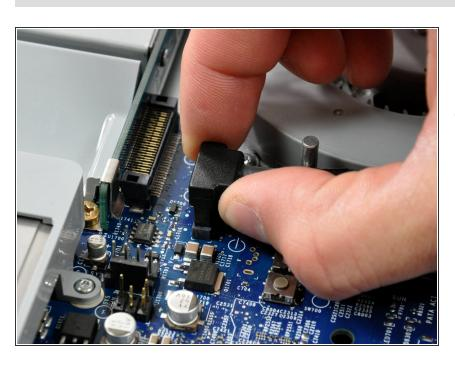
Disconnect the SATA data cable by pulling its connector straight up off the logic board.
