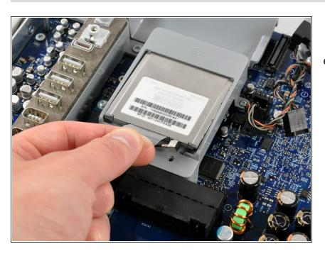
Lift the AirPort card slightly by its plastic tab and pull it straight away from its socket.
