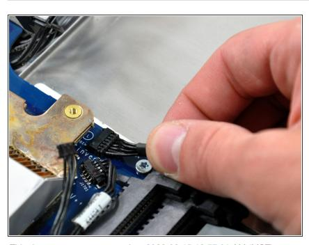
Disconnect the black inverter cable from its socket on the logic board by pulling the cable straight away from its socket toward the side of the iMac.
