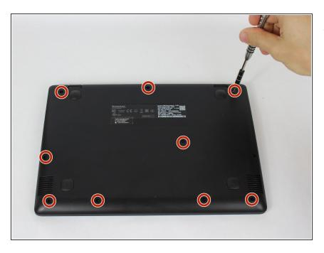
Use a #0 Phillips screwdriver to remove the nine 6mm screws from the larger back plate.
