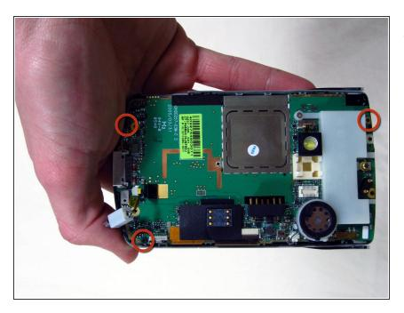
Use a 00 Phillips screwdriver to remove the three small screws holding down the motherboard.
