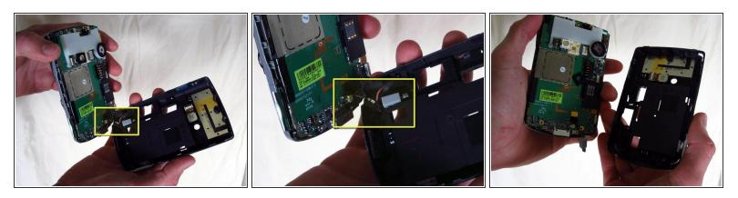
• Unplug the sensor wire that connects the two halves of the case before pulling the two halves apart. Not doing so will damage the sensor wire.
