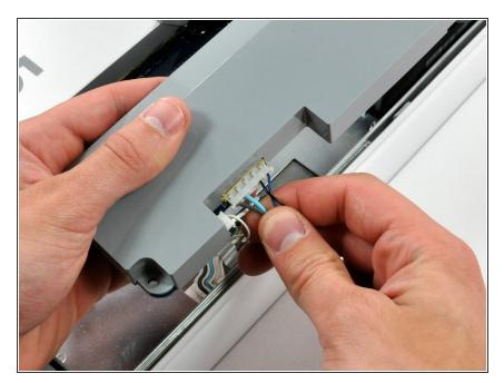
Disconnect the large inverter cable connector from the inverter by pulling straight away from its socket.
