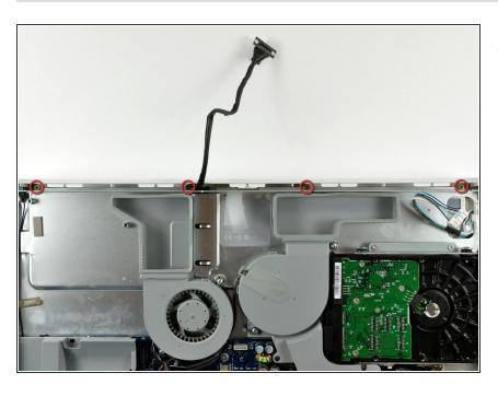
Remove the four coarse-thread 7.8 mm Phillips screws along the top edge of the iMac.
