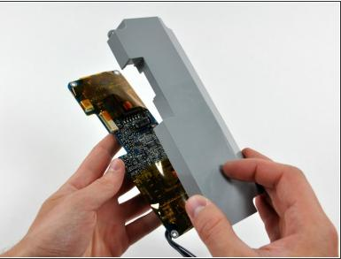
If you wish to replace just the inverter board, use a spudger to pry off its plastic cover.
