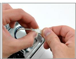
Remove the inverter cables from the inverter cable cover, and disconnect both connectors.
