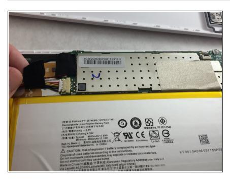
Remove the black piece of tape that is holding the red, yellow, and white wires in place.
