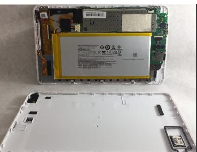
To remove the back panel, insert an opening tool into the small crack between the screen and back panel. Gently pry open the tablet.
