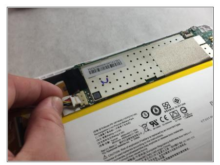
Once the tape has been removed, gently pinch the wires and remove them from the socket. They should come out easily.
