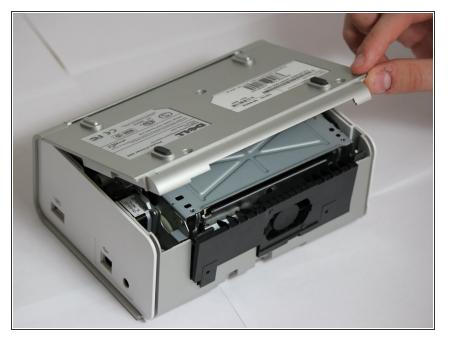
Rotate the photo printer so that the bottom panel faces up once again. Now lift off the bottom panel of the case to access all internal components.
