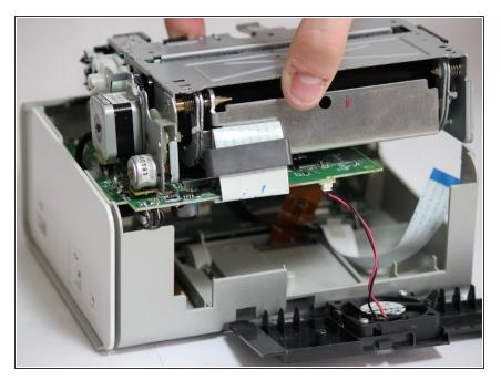
Carefully remove the inner components of the device by lifting the inner components up and out of the casing.
