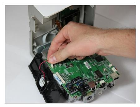
• Locate the red and black cable that is connecting the fan to the top of the logic board.
