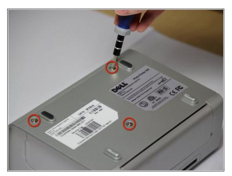
Use a Phillips #2 screwdriver to remove the three 5.65 mm screws on the bottom panel of the case in a counter-clockwise fashion.
