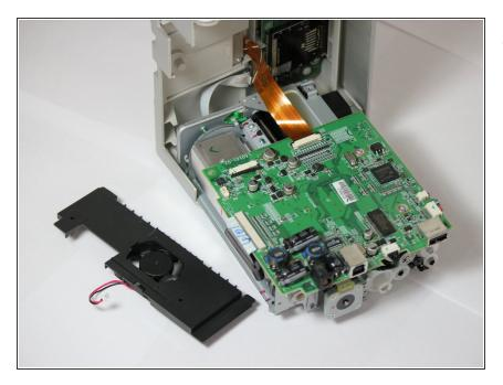
Carefully, remove the red and black cable from the logic board by pulling gently in order to isolate the cooling fan from the device.
