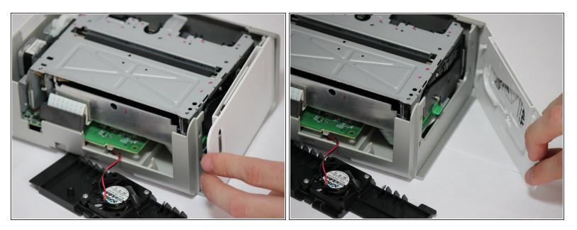
• Finally remove the side panel with the ink-cartridge door by holding the right side and pulling backwards with the left side.
