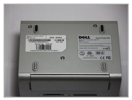
• Rotate the photo printer so that the bottom of the case faces upward.
