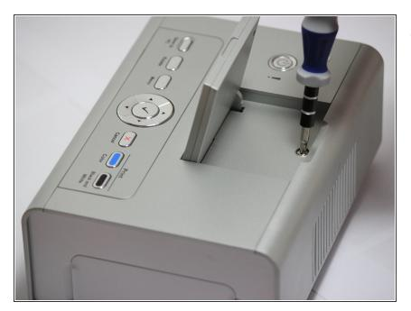
Rotate the device so that it is upright again. Under the LCD Panel there is a 9.62 mm screw, unscrew using a Phillips #2 screwdriver.
