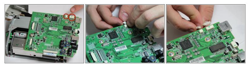
Locate the clips with multi-colored wires that connect the motherboard to the printing unit.
