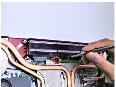
Unscrew the single 5.5mm Phillips #1 screw keeping the battery secure.
