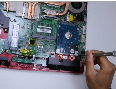
Remove the two 5.5mm screws with the Phillips #1 screwdriver.
