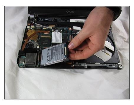
Hold the hard disk drive on the side where the brown clip was attached and lift it upwards to pull it out.
