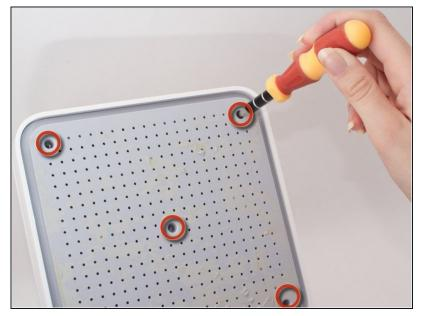
After removing the rubber covering, unscrew the five 4.9mm Phillips screws in the holes of the plastic casing.
