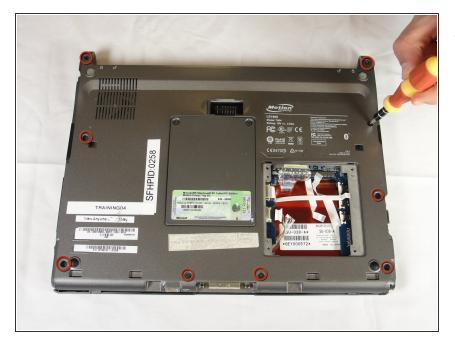
With a Phillips #1 screwdriver, Unscrew the nine 10mm screws holding the case together.
