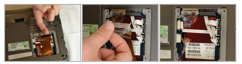
• Pull clear plastic tab to detach hard drive from tablet.
