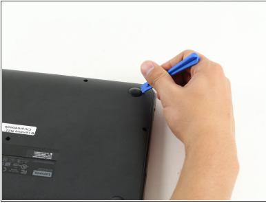
Wedge the plastic opening tool between the rubber foot and the bottom of the chromebook. Lift up
