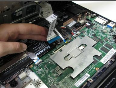
Disconnect the keyboard ribbon cable by lifting the ZIF connector lock with a plastic opening tool or fingernail and gently pulling the ribbon cable straight out of its socket.
