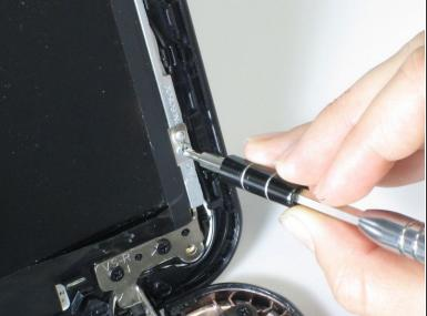
Remove the four 3.0mm Phillips screws symmetrically placed on either side of the screen.
