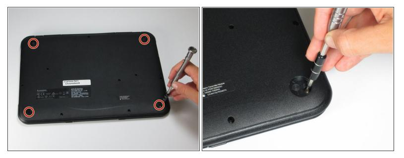
• Use a screwdriver to remove the four 5.0mm Phillips screws located under the rubber soles.
