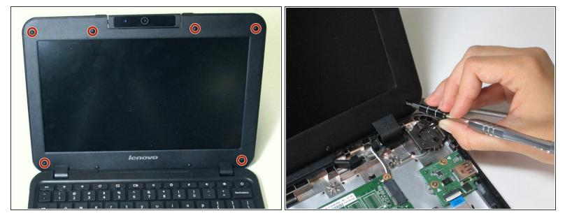
• Remove the six 4.0mm Phillips screws that are underneath the rubber pads with a screwdriver.
