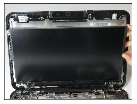
Remove the screen from the device.
