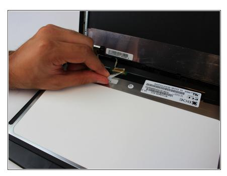
Gently remove the adhesive tape from the back of the screen.
