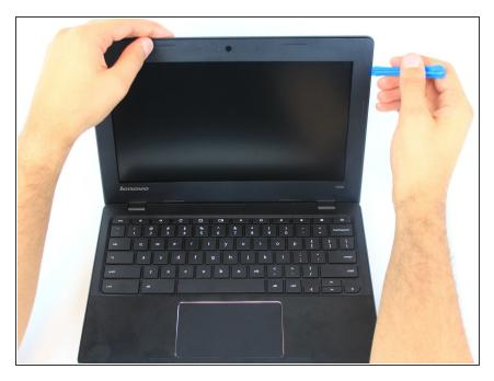
Use the plastic opening tool on the recessed notch to gently pry each side of around the screen up.
