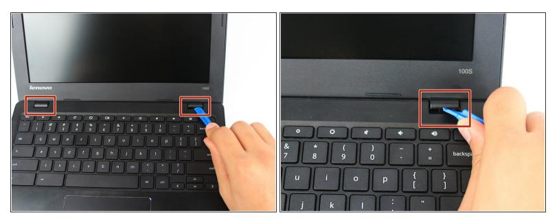
Carefully pry up and underneath both the (left & right) hinges of the screen cover.
