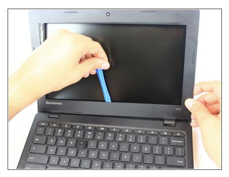
Use the opening tool on the inside of the screen plate and again on the sides to gently remove it.
