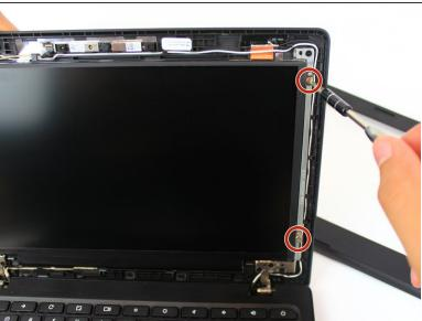
Use the #0 Phillips screwdriver to remove the four 6mm screws from the screen.
