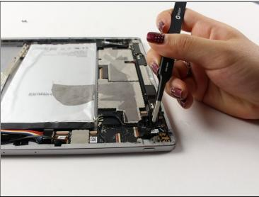
• Use <u>tweezers</u> to slowly pull up on the power button technology as far as possible without pulling out the two black wires attached.
