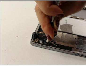
• Locate and remove the three 4.2mm Phillips #000 screws at the base of where the second wire is still connected.
