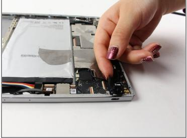
• Detach the larger connector wire by flipping the copper hinge located at the base of the connection with your fingernail.
