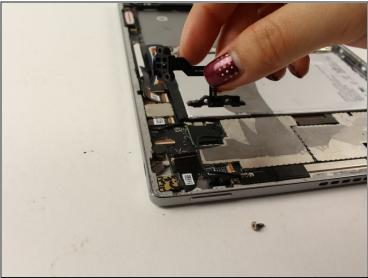
• Once all the screws are removed, gently pull up on the entire power button technology piece, to remove it from the device.
