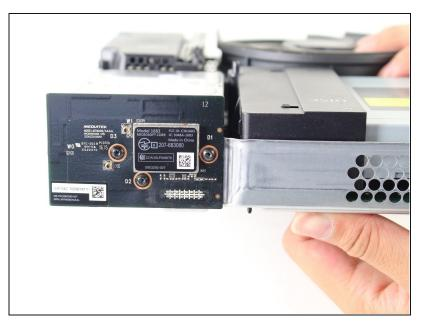
Search the sides of the interior case for the Wi-Fi card. It should be across from the hard drive.
