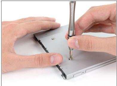
Use two Phillips #1 screws to secure the drive to its enclosure.
