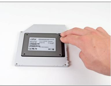
Once the hard drive is snug, reinsert the plastic spacer while holding the hard drive against the bottom of the enclosure.
