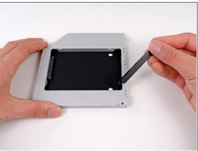
Remove the plastic spacer from the optical bay hard drive enclosure by pressing in on one of the clips on either side and lifting it up and out of the enclosure.
