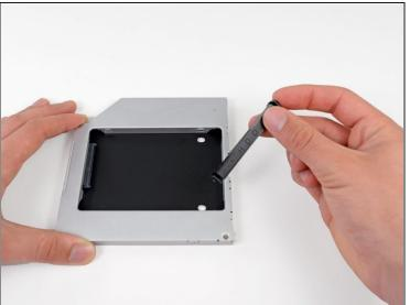
Remove the plastic positioner from the optical bay hard drive enclosure by pressing in on one
